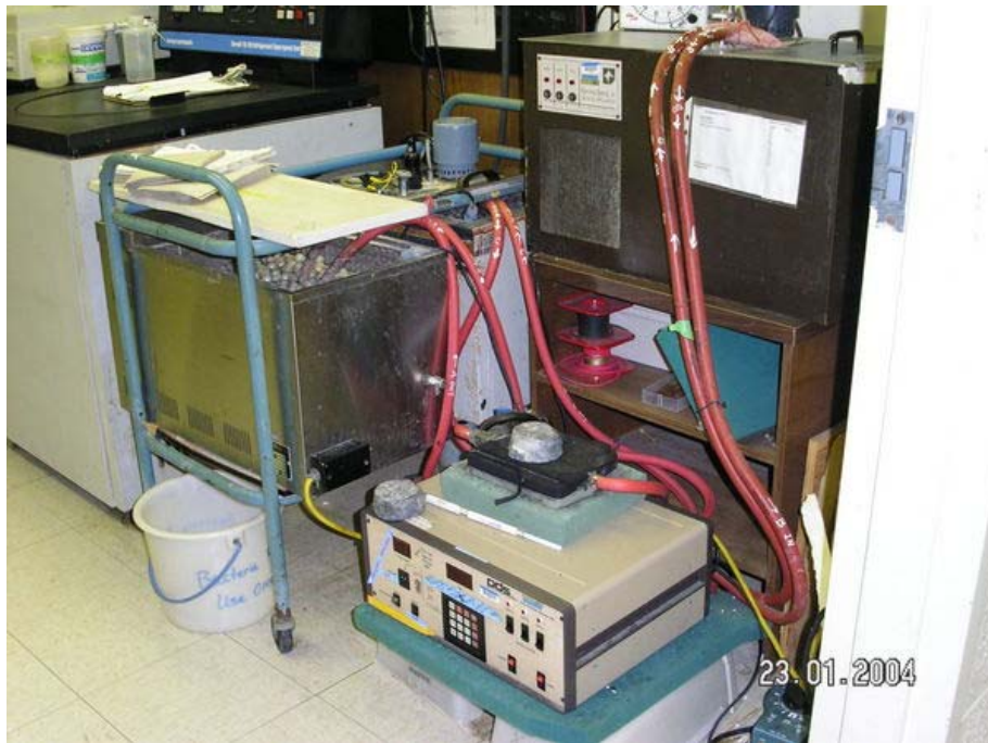
Figure 4. 20-year-old hand-made thermocycler (PCR machine) developed by Oliver in our laboratory.
